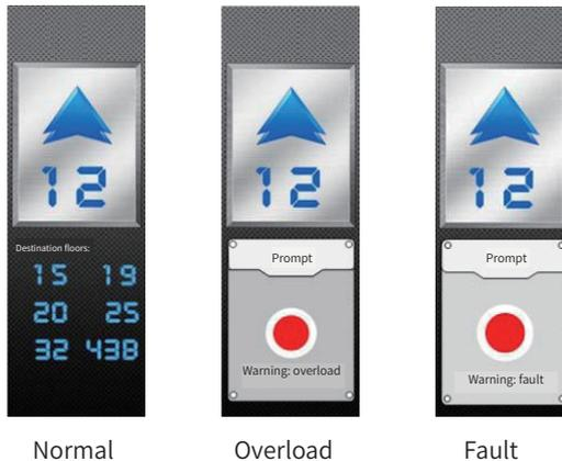
Figure 2-4 Examples of the car display interface
